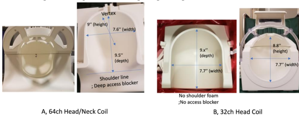
Figure 1. Inside dimension of 64ch and 32ch coil. The geometry of 64ch coil inside is a little formed to head shape with shoulder form, while that of the 32ch coil is simple cylindrical shape with half sphere cap. This difference makes positioning of a head positioning different for two coils.
